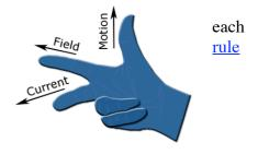
**Fleming's right hand rule** (for <u>generators</u>) shows the direction of <u>induced current</u> flow when a <u>conductor</u> moves in a <u>magnetic field</u>.
